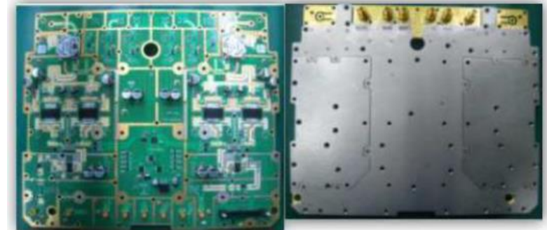
Copper & Aluminum Combined with Sweat-soldering
