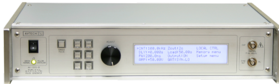
A high voltage pulse generator
