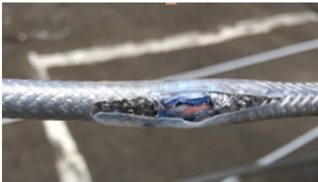
Exposed twisted wires to water
