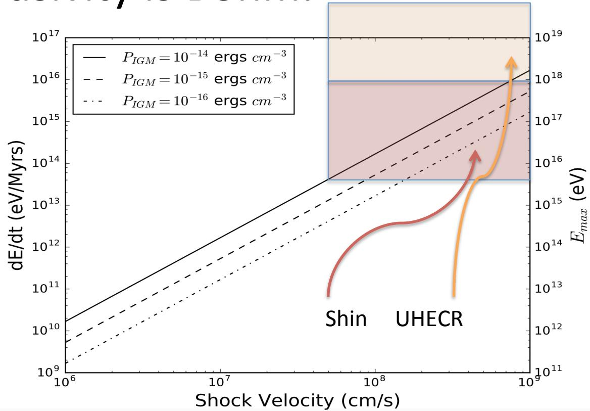
$$\frac{dE}{dt} = (1.5 \times 10^{-18} Z) \sqrt{4\pi P_{\text{IGM}}} V_{\text{shock}}^2 \quad \text{GeV/s}$$
