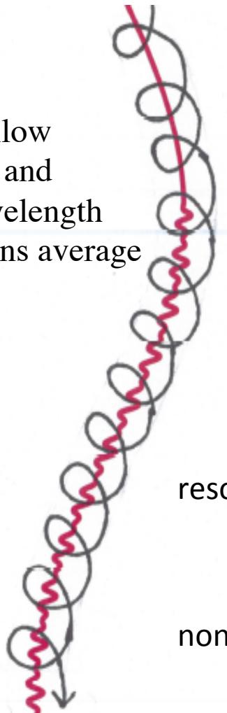
$$\omega - kv\mu = \pm\omega_c;$$
