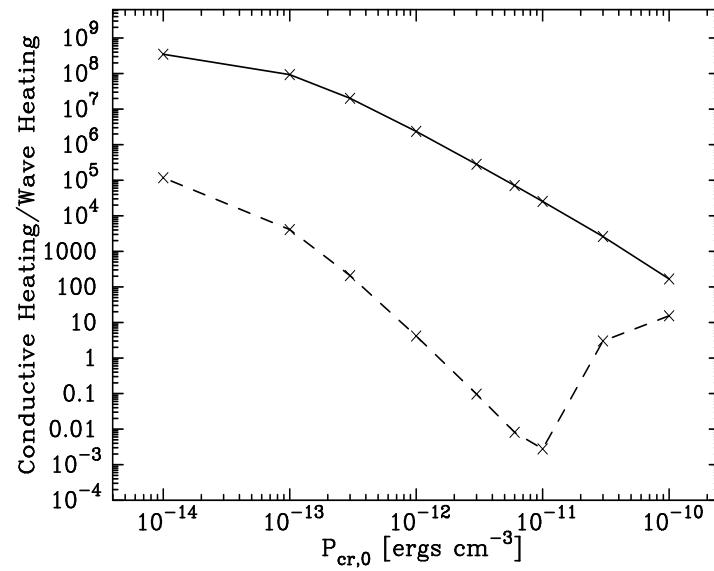
Ratio of conductive to wave heating in the model cloud. The upper & lower curves show maxima & minima, respectively. In the left figure  $B$  is varied, in the right figure  $P_{cr}$  is varied. Only a thin skin is heated, then cosmic rays decouple. From Everett & Zweibel 2011.
