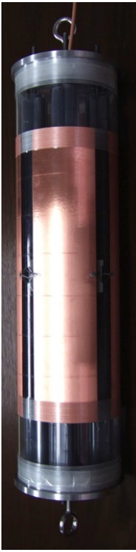
Antenna for horizontally polarized radio (Hpol antenna)
