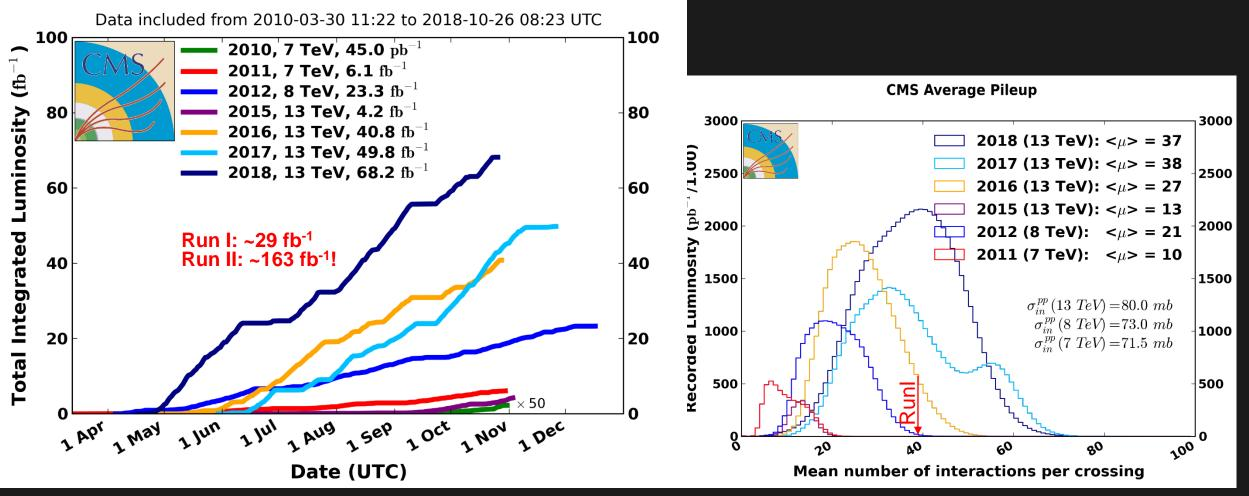
• LHC has delivered ~163 fb<sup>-1</sup>, CMS has collected data with >94% recording efficiency with a data certification ~90%.
