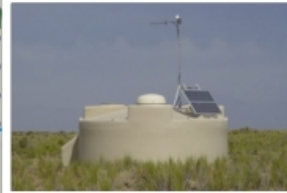
1665 surface detectors: water-Cherenkov tanks (grid of 1.5 km, 3000 km 2 )
