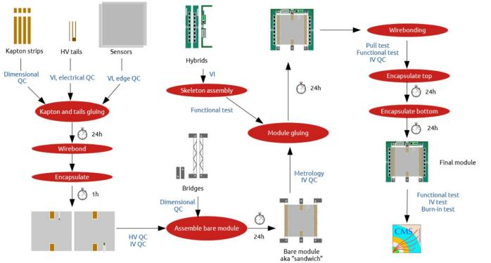
✓ Except for the actual assembly itself, the process includes multiple validation and qualification control tests
