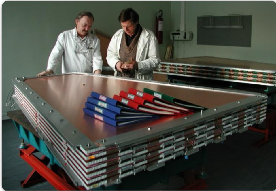
Open ME2/1 CSC being inspected at PNPI
