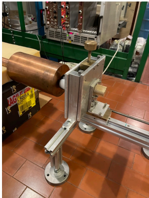
HPGe characterization with sources at STELLA (LNGS)
