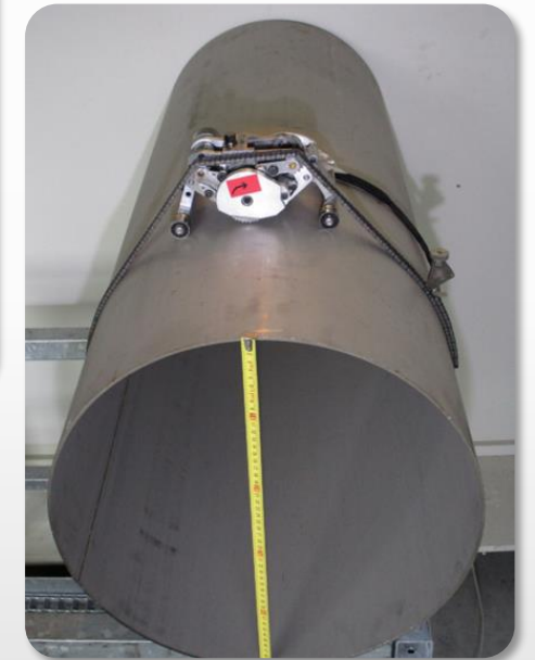
Example of light and compact orbital milling machine developed at CERN for pipe cutting. Credits: CERN
