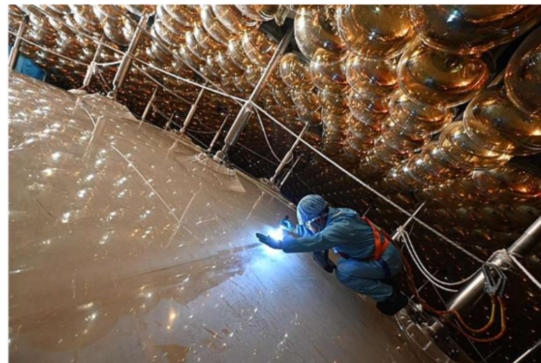
The central acrylic sphere and PMTs. Credit: JUNO Collaboration
