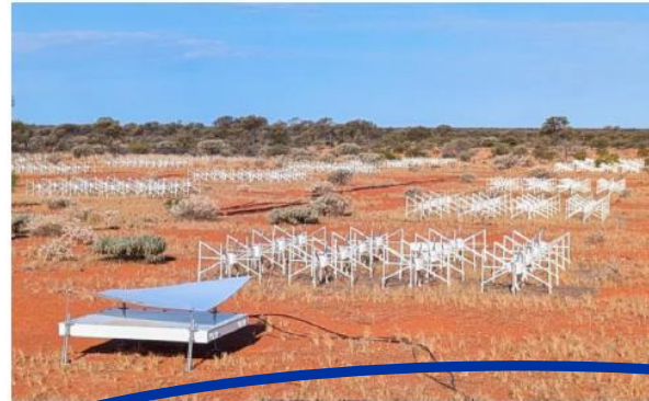
8-station prototype array installed at Murchison Widefield Array
