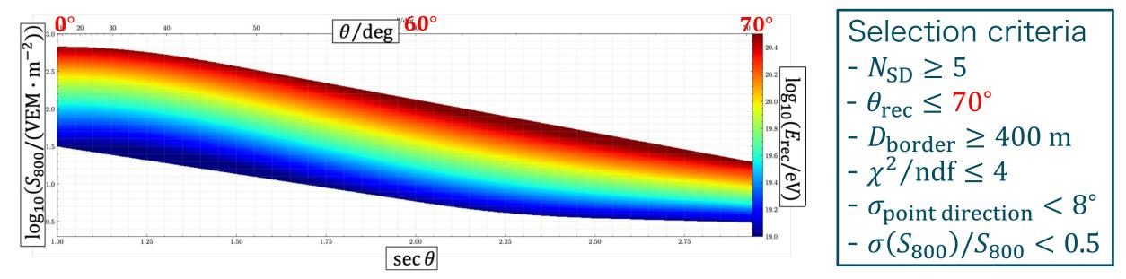
This extended table for the TA×4 SD enables the energy reconstruction of the primary cosmic ray in the range from Odeg to 70deg in zenith angle.
