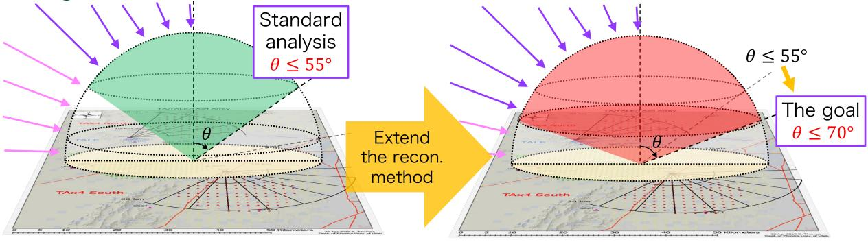
If extended from 55deg to 70deg, ~1.3× aperture of surface detector array
