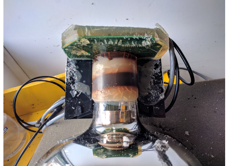
Auger XP1805 with potting silicone and nick
