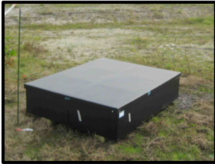
LORA LOFAR Radboud Array scintillator detectors
